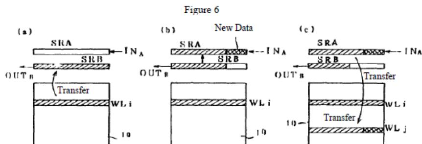
Figure 6 depicts shift registers SRA and SRB being used to transfer data from cells in a selected row WL<sub>i</sub> in memory array 10, to different cells in the selected row
