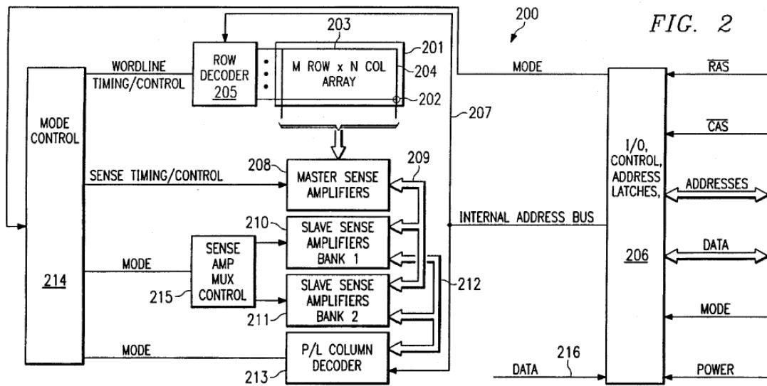
Figure 2 depicts a block diagram of memory system 200 with an  $M \times N$  array of flash memory cells 201, with wordlines (rows) 203 and bitlines (columns) 204. *Id.* at 5:52–57, 3:25–26. Representative memory cell 202 is located at the
