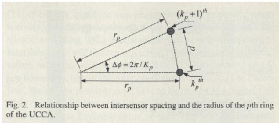
*Figure 1 of Chan illustrates a uniform concentric circular array (UCCA) with  $p$  rings. Figure 2 of Chan illustrates the relationship between intersensor spacing and the radius of the  $p^{\text{th}}$  ring of the UCCA.*
