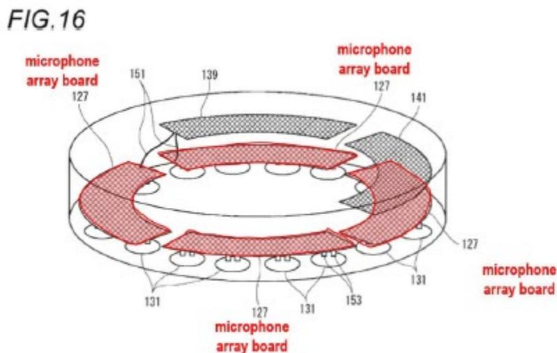
*Figure 16 of Sawa is a schematic diagram illustrating a microphone array structure including four microphone boards 127.*
