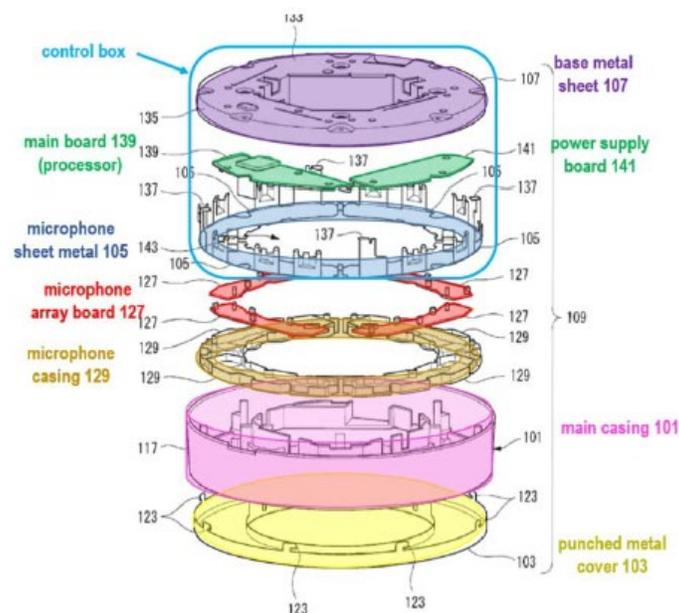
*Figure 12 of Sawa is an exploded perspective view illustrating a casing structure of microphone array 20.*
